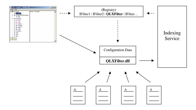
The Design tool let you create multiple filter descriptions. Each description is assigned an individual indexing condition. The condition is used by the filter dll to "probe" an xml file during the file scan. The file is indexed with a particular filter description only when the probing passed successfully the condition. In this respect, it is possible to scan xml files having the **same extension**, but totally **different xml content** and structure!
