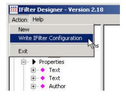
Within the last step, the filter configuration is written to the configuration file, the registry updated and the indexing service stopped and restarted. At this point, full-text queries and SPS dashboard site simple search ('contains' and 'freetext') will work.
